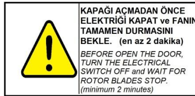
Figure 8.2. Electrical warning label
